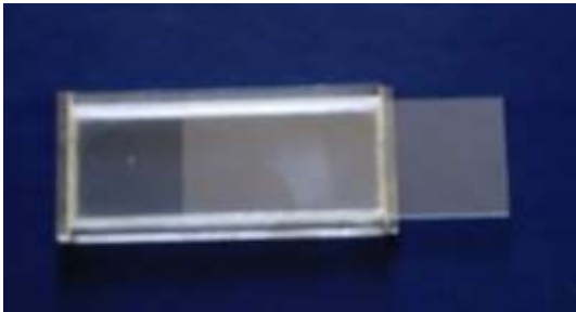
Fig. 3 “Pencil box” chamber for enumeration of ciliatoplankton.
